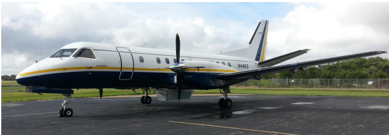
Figure 3. Saab 340 aircraft with the NRL MSAR radome mounted beneath the fuselage.
